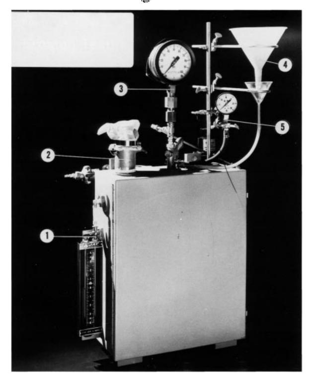
Note 1—Identified by number in this figure are: (1) cabinet pressure manometer, (2) dust collector vent, (3) test pressure gage, (4) grit feed tunnel, and (5) vacuum gage.
