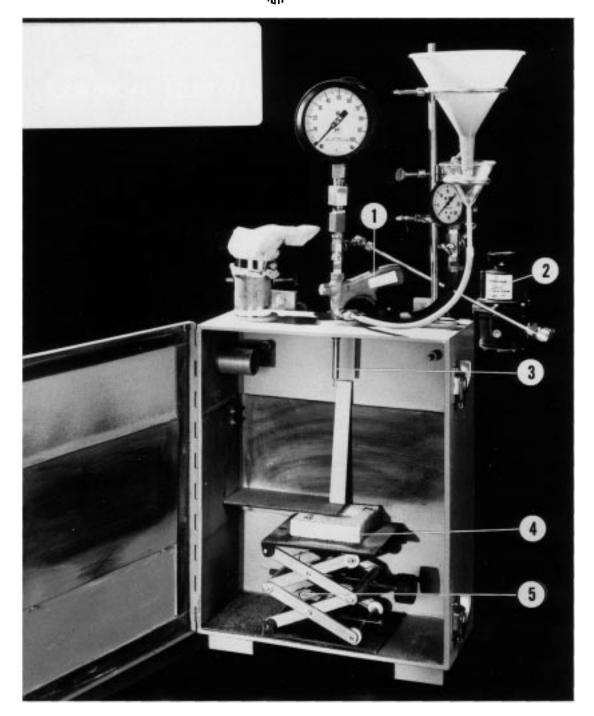
Note 1—Identified by number in this figure are: (1) sand blast gun, (2) air pressure regulator, (3) glass tube and metal stabilizing sleeve, (4) test sample, and (5) adjustable platform.
